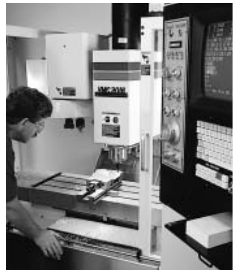
Rayite 100 media being machined on CNC-type milling equipment.
